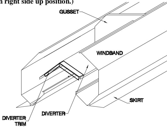
Form the Skirt Trim by hand so the 3/16" holes in the end (not the slots) match up with the holes in the ends of the skirts. Fasten to the skirts using 3/16" rivets.
