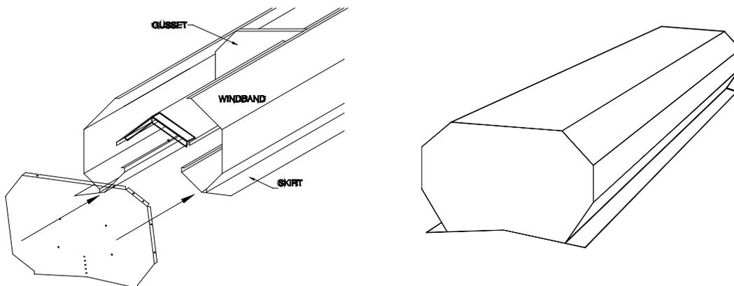
**Caulk the Skirt Trim and skirt/end cap joints using the polyurethane caulking.**
