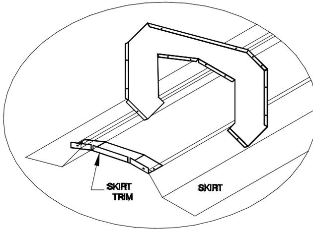
Attach the End Caps to the end of the vents with the windbands overlapping the flanges on the endcaps. Fasten using 1/8" rivets. Attach skirt and diverter trims to the end caps.
