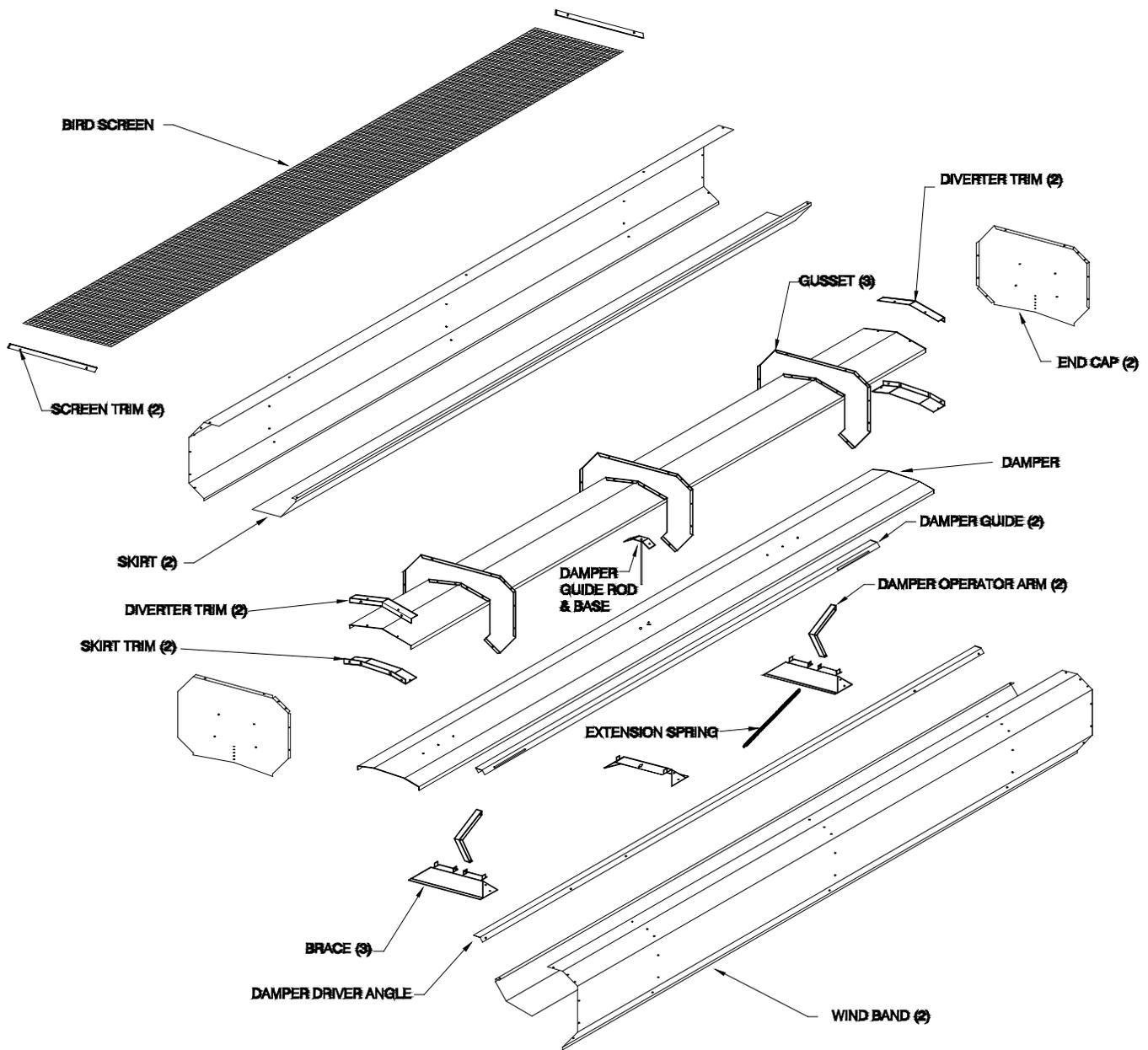
Lay the three gussets on a table with all 3 pieces facing the same direction spaced about 3 feet apart. Lay the diverter on top of the gussets. Tip the gussets up one at a time with the "horseshoe" facing up and fasten the diverter to the gussets with 1/8 X 1/8 ALUMINUM/STEEL POP RIVET WITH CLOSED END PART#AB42CLD (RV-9 only). For the RV-12 and up, use 3/16 X 1/4 ALL ALUMINUM POP RIVET WITH CLOSED END PART#AD64AH. Six rivets required.
