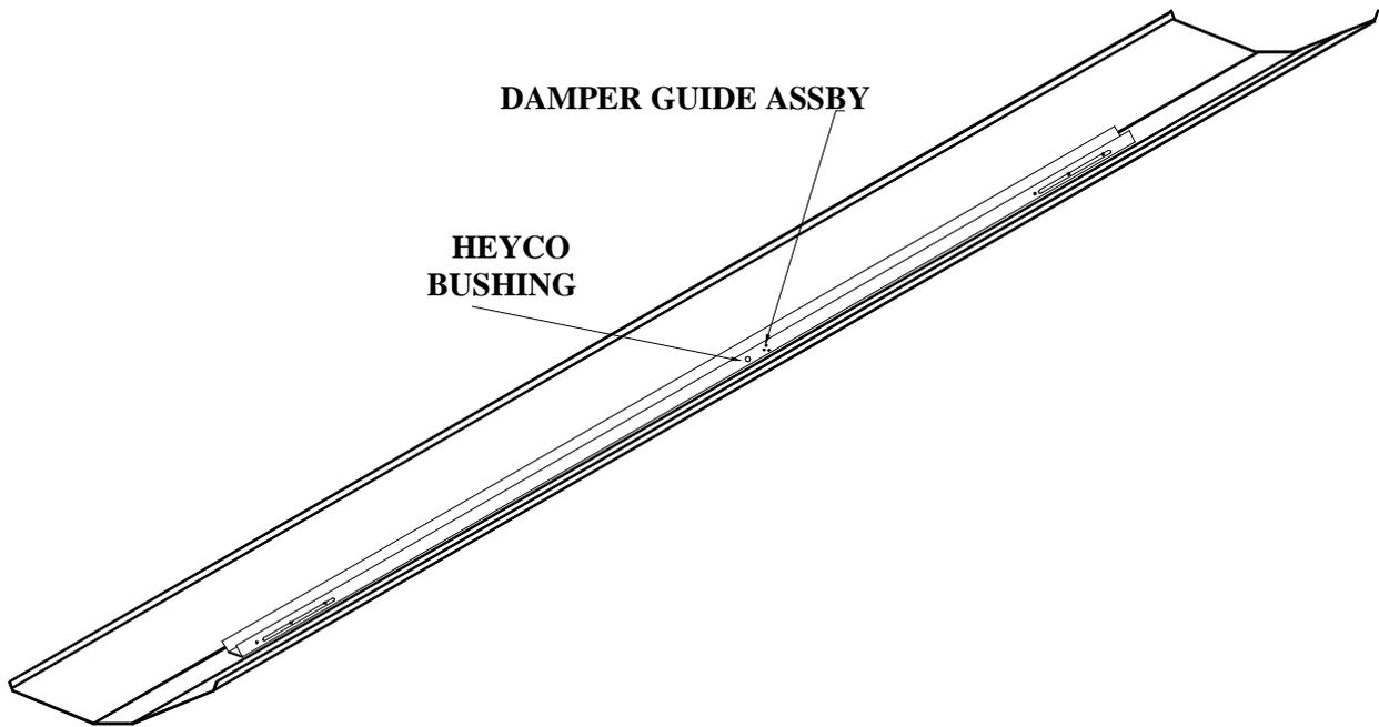
**Place damper assembly over guide rods and diverter.**
