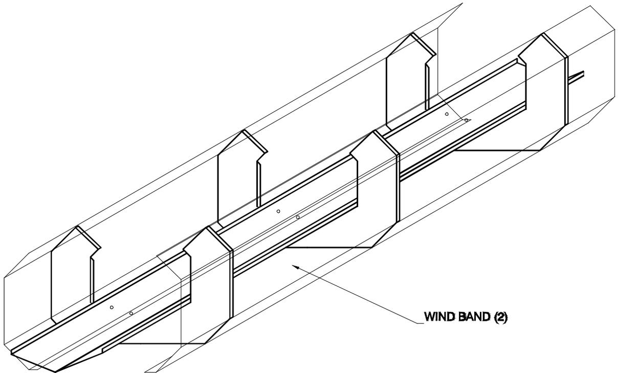
Lay the two skirt flashings on top of the gussets making sure the holes line up properly as shown below (windbands omitted for clarity).
