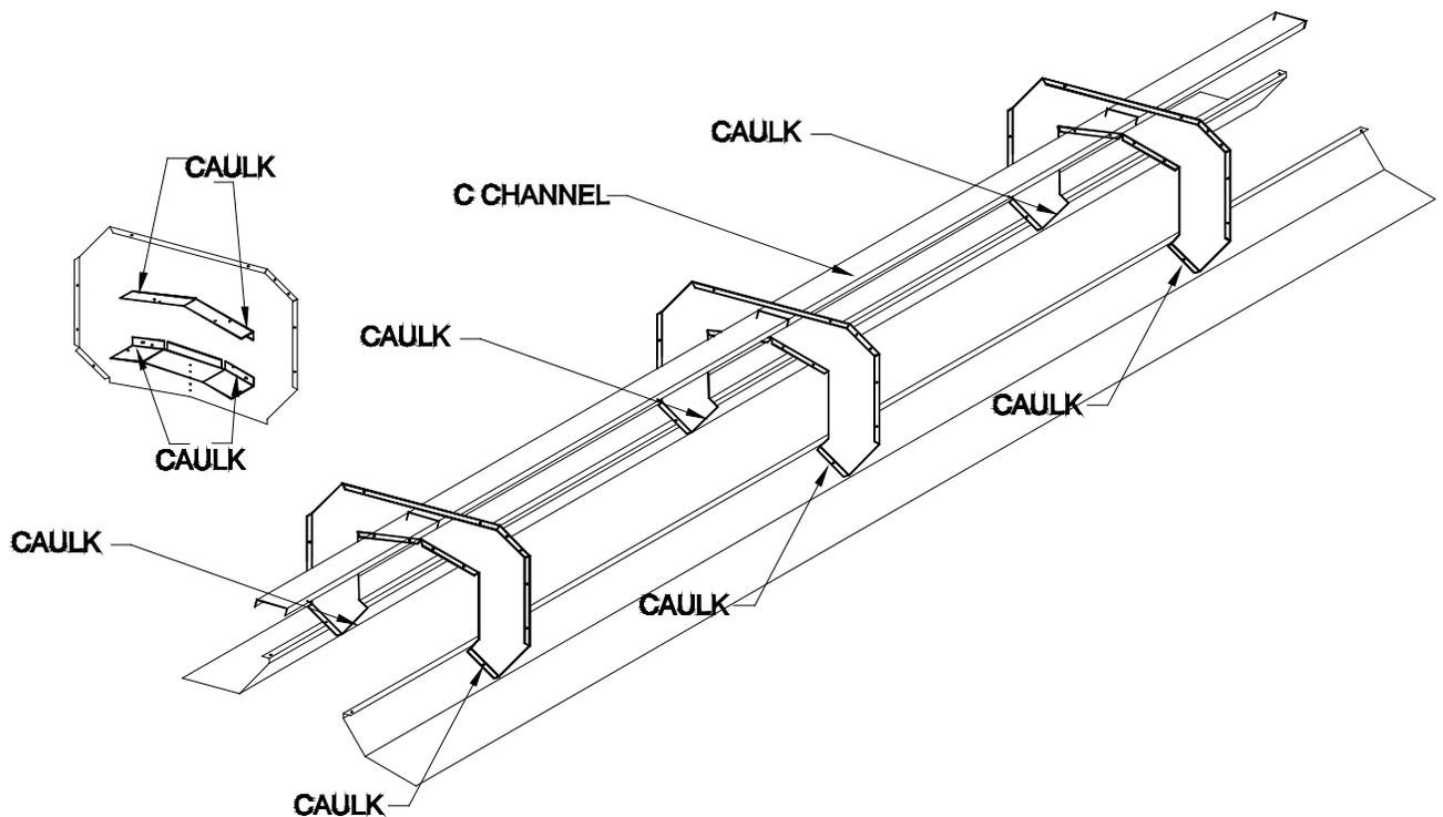
**Turn the vent over 180 degrees. Attach the C Channel lifting arm. Fasten to each gusset. Caulk the End Cap to the Diverter Trim using the polyurethane caulking.**
