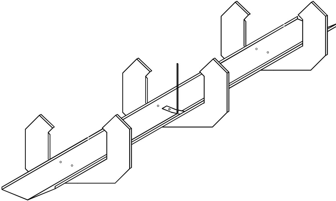
**Set up the damper with one Heyco guide rod bushing, and the one damper horizontal guide assembly. Use two 3/16 X 1/4 rivets PART#AB64A.**
