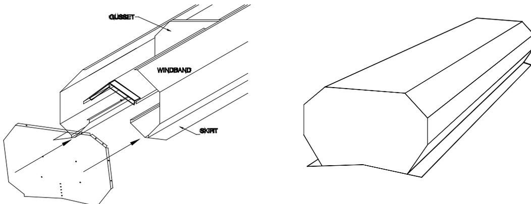
**RV9 and RV12 Models – Caulk the Skirt Trim using the polyurethane caulking.**
