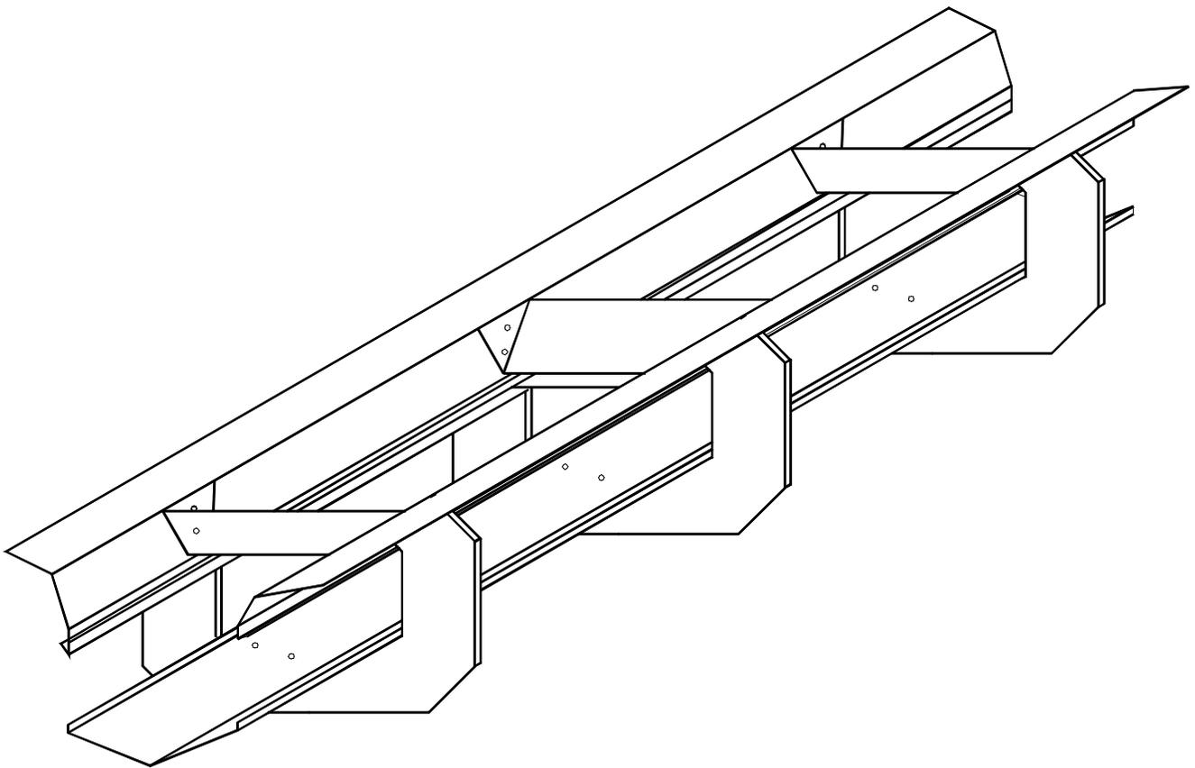
While in the up side down position, form the Diverter Trim by hand to match the shape of the water diverter and fasten one to each end of the diverter using 3/16" rivets. (Drawings shown in right side up position.)
