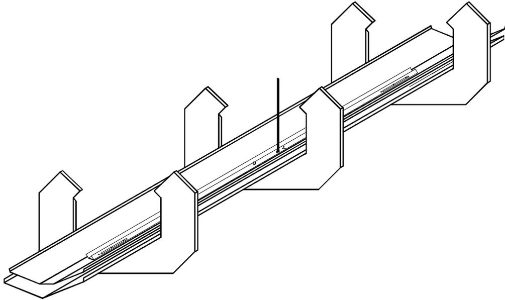
**Fasten the windbands to the sides of the gussets using 1/8" rivets. Do not fasten the windband to the braces near the bottom to allow the screen to be inserted.**
