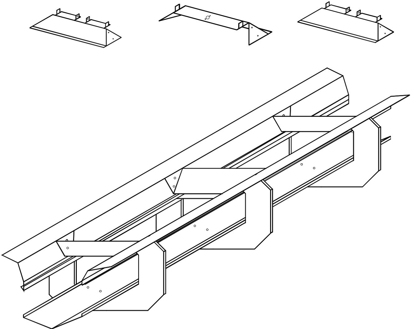
While in the up side down position, form the Diverter Trim by hand to match the shape of the water diverter and fasten one to each end of the diverter using 1/8" rivets. (Drawings shown in right side up position.)
